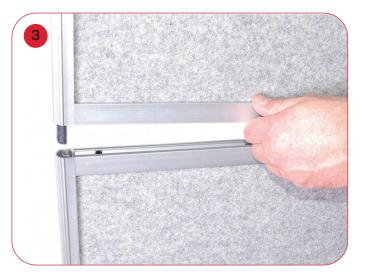
Attach the panels using the the black rubber connectors, simply place inside the hole
